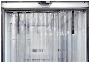
During picking of goods and when the goods are moved out of the truck body, the door curtains must remain closed completely. A door curtain reduce the air exchange with the environment, keeps the air temperature in the refrigerated body more constant and helps to prevent the entry of warm air from outside. Do not open the doors more often than necessary.
